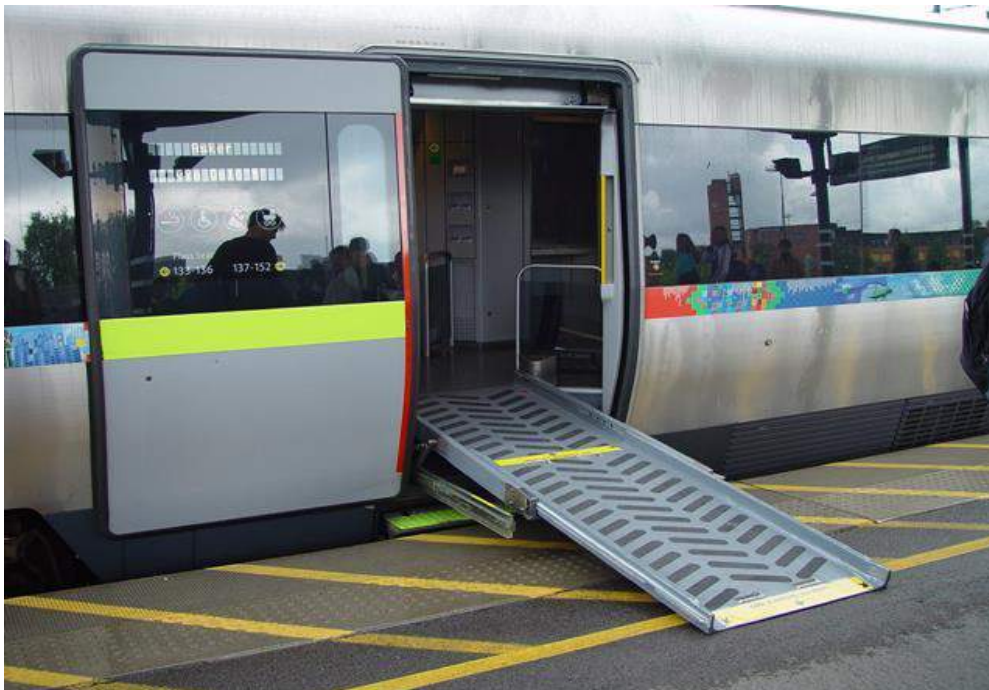
Figure 11-12: Retrofitting of ramp for sub-urban rail
