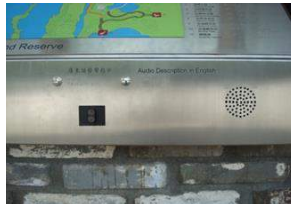
Figure 6-24: Speaker and buttons in talking signs
