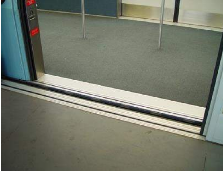
Figure 10-7: Level boarding in Delhi metro Rail Coach
