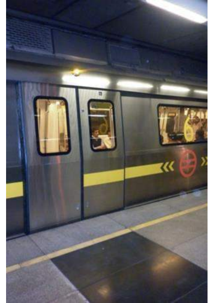
Figure 10-8: Warning strip on platform
